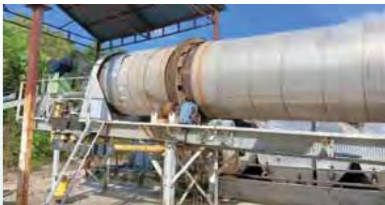
Pundut premix plant uses natural gas for its production
